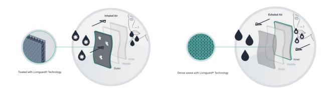
The middle layer is a non-woven industry standard filter according to EN 14683:2019 with a filtration efficacy of at least 95%.
